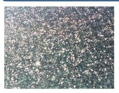
The black crackle finish, sometimes called 'wrinkle' or 'camera case' finish, is on MGB/C and Midget dashboards. It has a quiet elegance. The restrained, textured black sets off the chrome details and contributes an aviation appearance.
